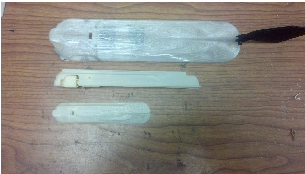
Figure C.1: A direct comparison among components of the 1, .75, and .5 scale models, in decreasing order of size.
