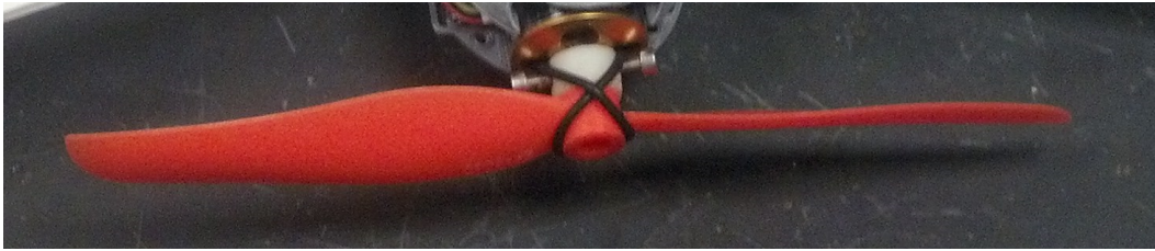
(a) The original, prop-saver, propeller mounting design.
